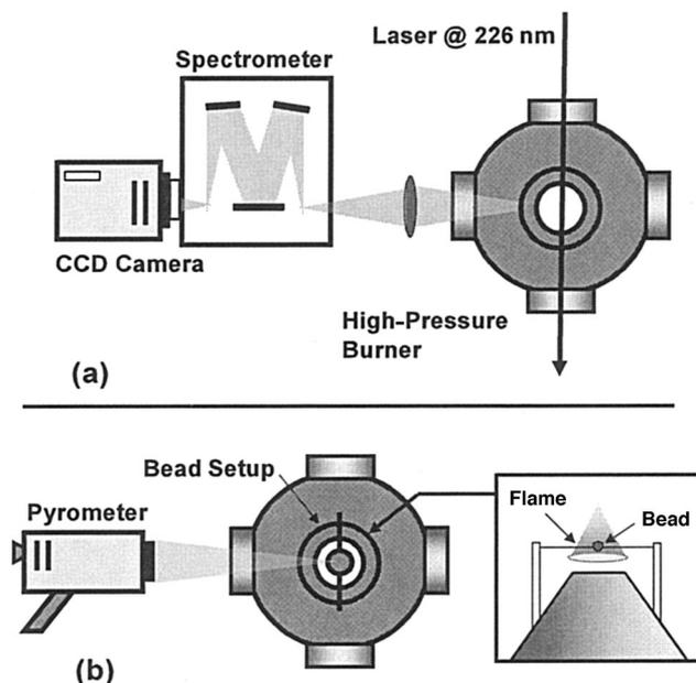
Fig. 5. Experimental setup (a) for NO-LIF multiline thermometry and (b) for an intrusive probe (Pt/Rh bead) infrared pyrometer measurement.
