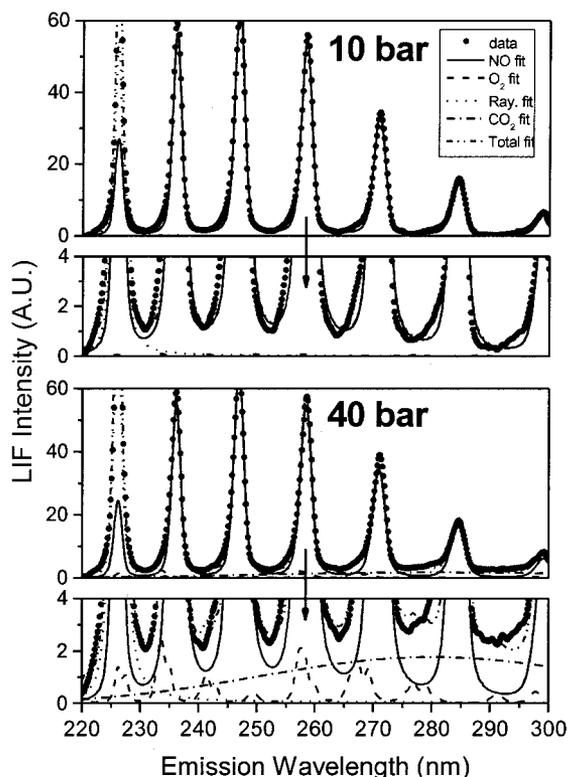
Fig. 8. LIF fluorescence spectrum with NO A-X(0, 0) excitation at 10 and 40 bars. The spectrum is separated into contributions from different components (NO, CO<sub>2</sub>, and O<sub>2</sub> LIF, Rayleigh scattering). The lower part of each plot is magnified for a clearer view of the spectral separation. The baseline is defined as sum of all signals in the detection region (230–310 nm), excluding NO LIF.  $\lambda_{ex} = 226.034$  nm (400 ppm NO seeding,  $\phi = 0.9$ ).
