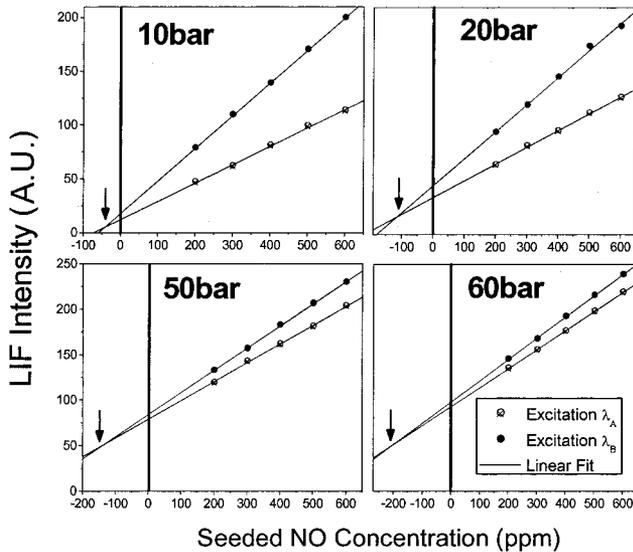
Fig. 10. NO addition plots for determination of baseline strength at 10, 20, 50, and 60 bars. Two lines in each graph are linear fits to the two different excitation wavelengths. Excitations A and B refer to two different excitation wavelengths ( $\lambda_A$ , 226.03 nm;  $\lambda_B$ , 226.042 nm).
