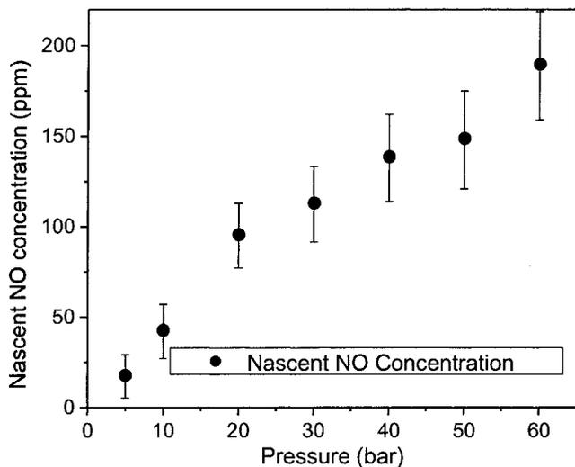
Fig. 13. Nascent NO concentration versus pressure. Concentrations are derived from the NO addition method.
