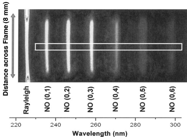
Fig. 6. Raw image, scan from a camera at an individual point of excitation ( $p = 20$  bars,  $\lambda_{\text{ex}} = 226.034$  nm). The white box in the center shows detection region for reconstruction of laser excitation spectrum (detection region is broadband 230–310 nm).
