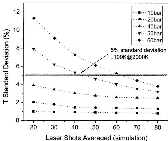
Fig. 4. Sensitivity analysis of temperature fitting with respect to the number of individual laser experiments that are averaged on a chip at each wavelength position for 2000 K. The scan range is 225.944–226.112 nm.
