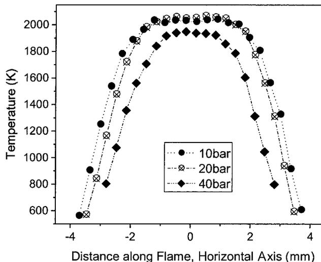
Fig. 14. Spatial temperature profile (1D) along a horizontal line in the flame (3 mm above burner matrix) for 10, 20, and 40 bars.  $\phi = 0.9$   $CH_4$ /air flame with 400 ppm NO seeding.
