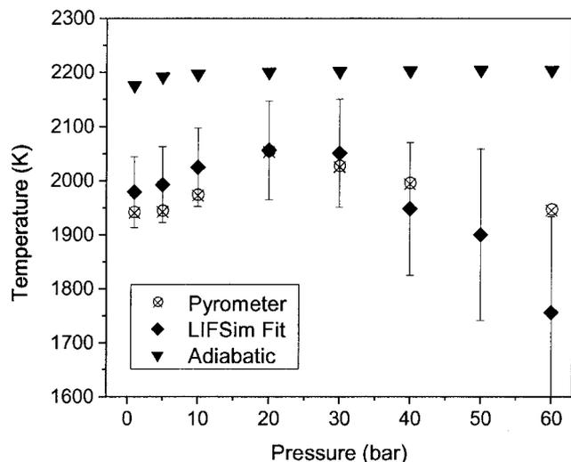
Fig. 12. Temperature versus pressure for the two different measurement techniques (multiline fitting, pyrometer). Adiabatic temperatures have been calculated by using the thermal equilibrium model (Stanjan<sup>37</sup>).
