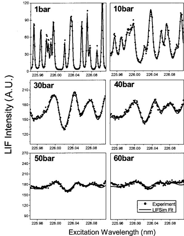
Fig. 11. Multiline temperature fitting in 1–60 bars,  $\phi = 0.9 \text{ CH}_4$ /air flames (NO seeding at 400 ppm). The LIF-intensity scales of the 30, 40, 50, and 60 bar figures have been magnified for viewing clarity.
