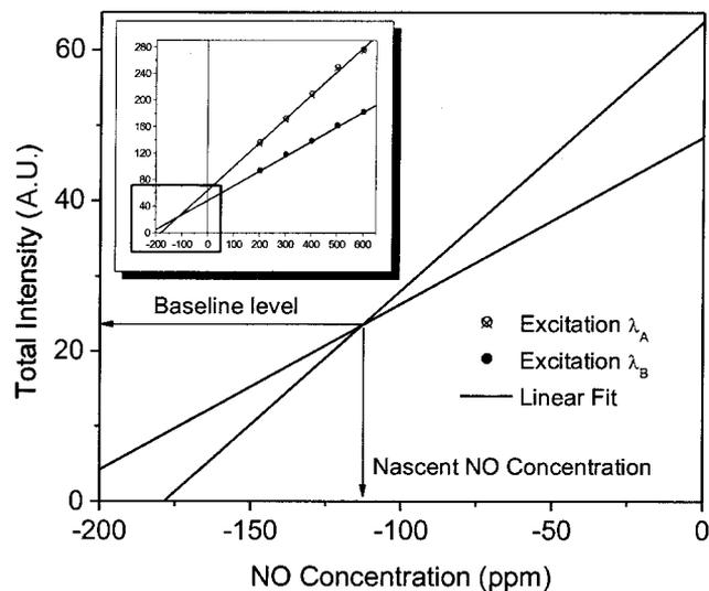
Fig. 9. NO addition method for the determination of the baseline strength and the nascent NO concentration at  $p = 30$  bars. The plot shows a magnified view of the small box in the inserted graph. The NO addition is varied from 200 to 600 ppm, and NO LIF is detected with excitation at two different wavelengths. Excitations A and B refer to two different excitation wavelengths ( $\lambda_A$ , 226.03 nm;  $\lambda_B$ , 226.042 nm).
