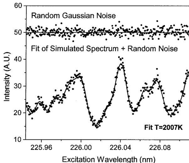
Fig. 2. Example of sensitivity analysis by using simulated spectra with added noise (Gaussian) and fitted to extract temperature at 20 bars (225.944–226.112 nm region). Random Gaussian noise is added to simulated spectra for temperature fitting to simulate experimental conditions.
