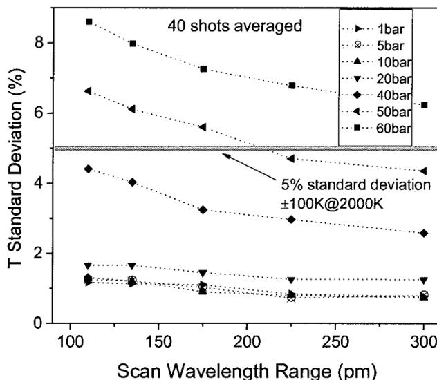
Fig. 3. Sensitivity analysis of temperature fitting with respect to scan wavelength range for 2000 K. The scan range centers around 226.03 nm (O<sub>2</sub>-LIF suppression region). The signal from 40 laser pulses is averaged on a chip for each individual data point.
