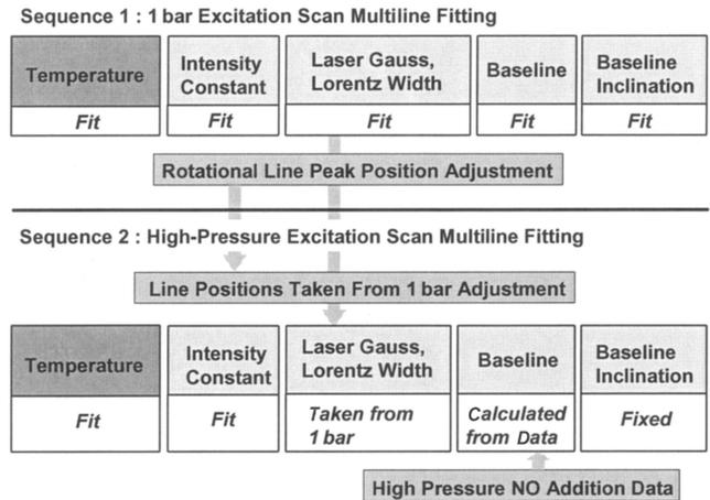
Fig. 7. Schematic of a multiline fit routine. Sequence 1 (upper) fits all parameters to determine the laser line shape and line positions. Sequence 2 (lower) extracts temperature with a reduced number of fit parameters.
