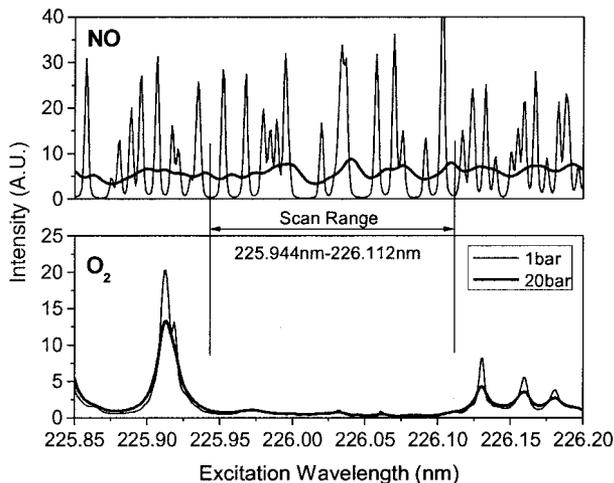
Fig. 1. Numerical simulation (LIFSim) of NO and O<sub>2</sub> LIF-excitation spectra in the range of 225.8–226.2 nm at 2000 K. The scan range (225.944–226.112 nm) is located in the region of minimum O<sub>2</sub> LIF interference. As spectra overlap caused by collisional broadening at 20 bars can be observed in the NO spectra, whereas O<sub>2</sub> is less affected because of predissociation. The intensities of NO and O<sub>2</sub> are on the same scale.
