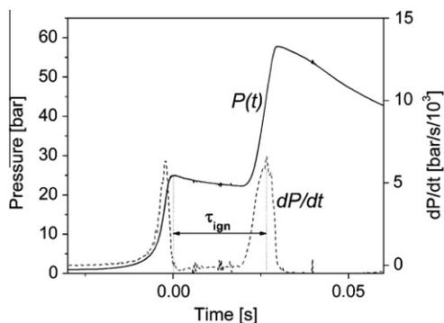
Fig. 4. Ignition delay definition. Reactive ethanol/air aerosol pressure trace  $[P(t)]$  and corresponding time derivative  $(dP/dt)$  used to calculate the ignition delay ( $\tau_{\text{ign}}$ ). Molar composition:  $\text{C}_2\text{H}_5\text{OH}/\text{O}_2/\text{N}_2 = 1.0/6.0/22.6$ . Conditions:  $P_0 = 1$  bar,  $T_0 = 343$  K, compression ratio = 14.2.
