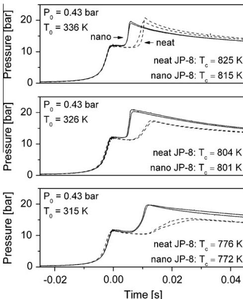
Fig. 7. Nanoparticle-enhanced ignition of JP-8. Reactive pressure traces for neat JP-8 (dashed lines) and for nanoparticle-enhanced JP-8 (solid lines). Molar composition: JP-8/O<sub>2</sub>/N<sub>2</sub> = 1.0/32.5/122.2.
