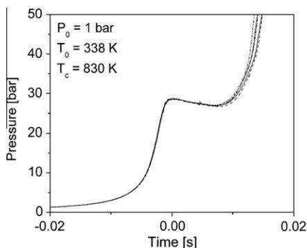
Fig. 5. Experimental repeatability. Demonstration of the experimental repeatability of autoignition of an ethanol aerosol charge at  $P_c = 28$  bar,  $T_c \approx 830$ . Molar composition (aerosol test):  $C_2H_5OH/O_2/N_2 = 1.0/6.0/22.6$ . Initial conditions:  $P_0 = 1$  bar,  $T_0 = 338$  K.
