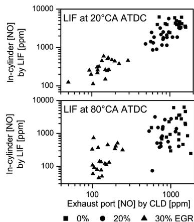
Fig. 12. Correlation of instantaneous NO-LIF concentrations (averaged over the imaged area) and exhaust port fast CLD measurements obtained from the corresponding working cycle. Note the double-log scale.
