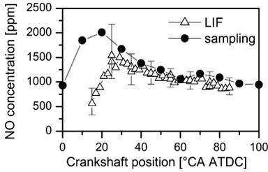
Fig. 8. Comparison of in-cylinder NO concentrations obtained with LIF and in-cylinder gas sampling. Homogeneous ( $\phi = 1.0$ ) engine operation at 0.3 MPa indicated mean effective pressure (IMEP), 2000 rpm, 0% EGR.
