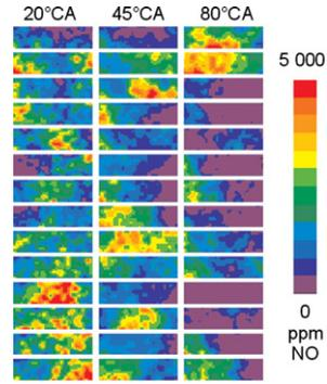
Fig. 9. Instantaneous NO concentration fields. Stratified ( $\phi = 0.4$ ) engine operation, 20% EGR, 2000 rpm, 0.3 MPa IMEP. The images show an area of 14 × 4 mm<sup>2</sup>.
