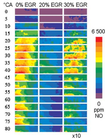
Fig. 10. Average NO concentration fields for different EGR ratio. Stratified ( $\phi = 0.3\text{--}0.5$ ) engine operation, 2000 rpm, 0.3 MPa IMEP. The images show an area of 14 × 4 mm<sup>2</sup>. At 30% EGR the look-up table is enhanced by a factor of 10.
