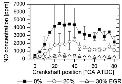
Fig. 11. Average NO concentrations from Fig. 10 for different EGR ratio.
