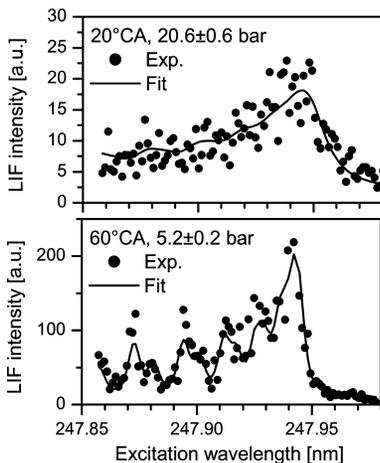
Fig. 4. LIF excitation scans in fired engine (homogeneous charge) and fits of simulated NO-LIF spectra to the experimental data.
