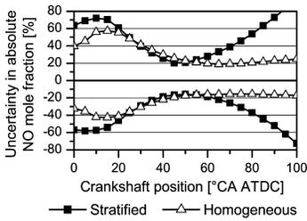
Fig. 7. Error analysis of NO-LIF quantification for stratified and homogeneous engine operation.
