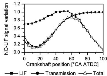
Fig. 5. Signal variation of a fixed NO concentration (stratified engine operation) versus crankshaft position and its contributions from LIF signal yield (normalized to 40°CA) and attenuation correction. The calibration (1900 K, 1 bar) condition corresponds to a LIF factor of 2.1 on this scale.
