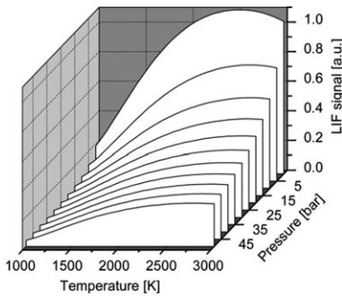
Fig. 1. Simulated NO-LIF signal strength versus temperature and pressure with excitation at the A–X(0,2)  $O_2$  bandhead at 247.94 nm, normalized to 1 bar, 2000 K.
