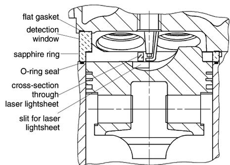
Fig. 2. Optically accessible four-cylinder engine with realistic piston and combustion chamber geometry.
