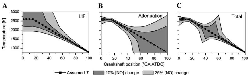
Fig. 6. Temperature sensitivity of NO-LIF quantification (stratified engine operation). Shown are the temperature values used in the data evaluation versus crank angle. The gray areas correspond to the temperature range that would result in a  $\leq 10$ (25)% change in evaluated NO mole fraction. (A) LIF signal yield, (B) laser and signal attenuation, and (C) total  $T$ -sensitivity.
