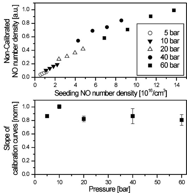
**FIGURE 4** Calibration by NO seeding: The upper plot shows the linearity of the NO signal intensity versus NO seeding concentration at 5, 10, 20, 40 and 60 bar. The slopes of the resulting linear fits yield the calibration information and indicate the over-all NO-LIF yield. The lower plot compares these data with the results of spectra simulations taking into account all  $T$  and  $p$ -dependent terms of (1)
