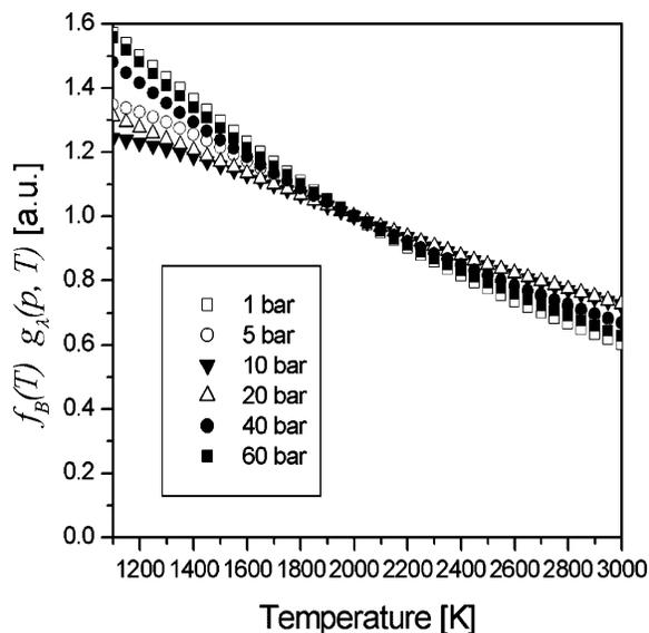
**FIGURE 1** Simulated temperature-dependence of the NO-LIF excitation efficiency for the  $A - X(0, 0)$  transition used in this work. The calculation includes the variation of the population of the laser-coupled level in the ground state and the overlap function  $g_\lambda$ , normalized at 2000 K
