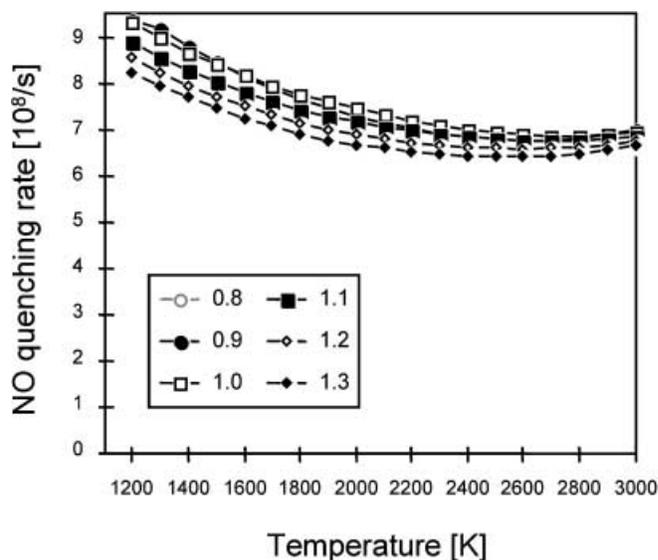
**FIGURE 2** Temperature-dependence of the NO-LIF quenching rates in equilibrium burnt gases at fuel/air ratios from 0.8–1.3 at 10 bar (methane/air flame). Temperature-dependent quenching cross-sections are taken from [23]
