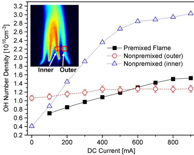
Fig. 4. OH number density with the same flow conditions (total flow rate is 9 SLPM, and  $\phi = 0.95$ ) but different currents for both premixed (from data point, the same as in Fig. 3) and nonpremixed (two data points, one is the outer flame front and the other is the inner flame front) flames.
