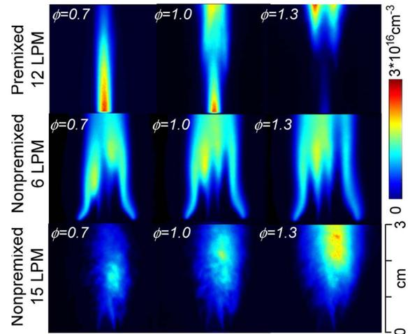
Fig. 5. (Top) Averaged OH PLF images for all flow rates at premixed mode with  $\phi = 0.7, 1.0,$  and  $1.3$ . Averaged OH PLF images for (middle) 6 LPM and (bottom) 15 LPM at nonpremixed mode with  $\phi = 0.7, 1.0,$  and  $1.3$ .
