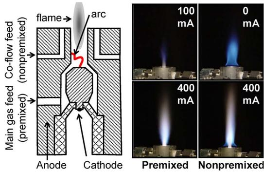
Fig. 1. (Left) Schematic of transient arc plasmatron with cathode in the center and two different inlets are used to get two different experimental setups. Images for premixed (100- and 400-mA dc currents) and nonpremixed (0 and 400-mA dc currents) flames of methane/air with equivalence ratio of 0.9.
