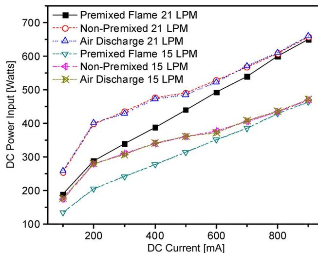
Fig. 7. DC power input with different current for air plasma, premixed flames, and nonpremixed flames.
