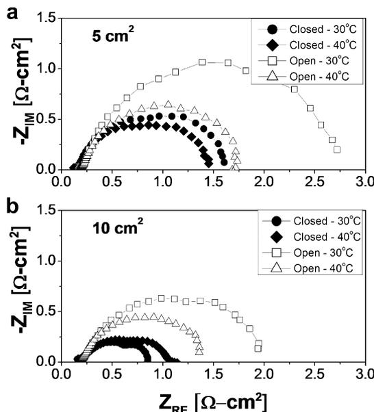
**Fig. 8.** Nyquist curves at 0.4 A/cm<sup>2</sup>. (a) 5 cm<sup>2</sup> open and closed cathode (b) 10 cm<sup>2</sup> open and closed cathode.
