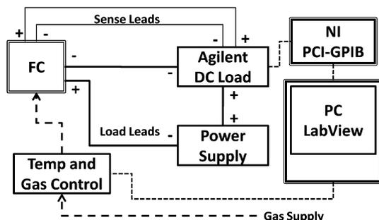
Fig. 3. Test setup for fuel cell operation.
