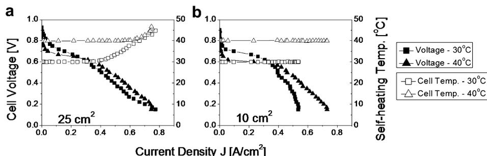
Fig. 4. Polarization curves for the a) 25 cm<sup>2</sup> and b) 10 cm<sup>2</sup> open cells. Right axis shows cell temperature. Self-heating is evident for the 25 cm<sup>2</sup> open cell in a).
