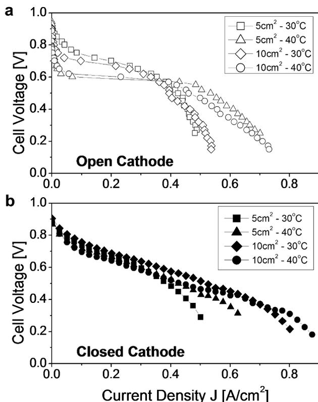
Fig. 6. Polarization curves at 30 °C and 40 °C. (a) Open cells (b) Closed cells.
