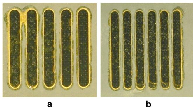
Fig. 7. Water accumulation on the GDL of open cells at 30 °C and 0.4 A/cm<sup>2</sup>. (a) 5 cm<sup>2</sup> cell (b) 10 cm<sup>2</sup> cell.
