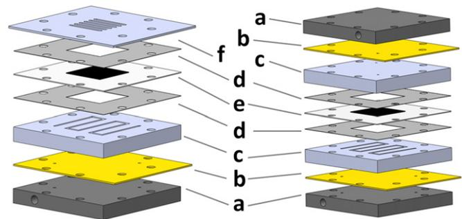
Fig. 1. Exploded view of the open-cathode, air-breathing fuel cell (left) and closed fuel cell (right).
