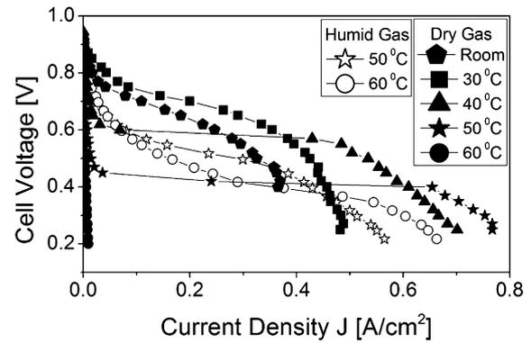
Fig. 5. Polarization curves for a temperature scan of the 5 cm<sup>2</sup> open cell.
