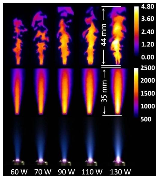
Fig. 5. Images of (top) OH number density [ $10^{16}$   $cm^{-3}$ ], (middle) averaged temperature (in degrees Kelvin), and (bottom) plasma-coupled combustion discharge at varying microwave power levels, increasing left to right. The total flow rate is 15 l/min at an equivalence ratio of  $\phi = 1$ .
